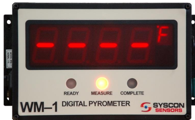
Figure 5: On-going temperature measurement indicated by Yellow (Measure) light and four dashes on the display
