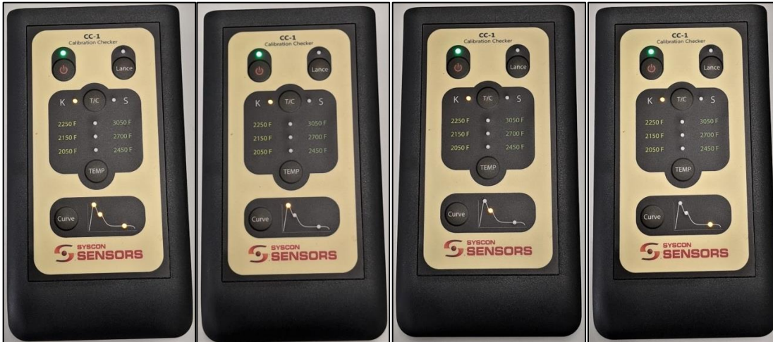
Figure 15: CC-1 panel showing the progression of the cooling curve test
