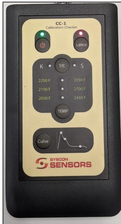
Figure 13: Lance check when insulation is less than 1M\Omega
